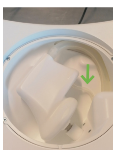
Push the small hose to straighten it
