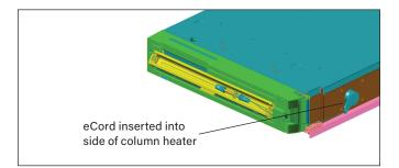
Figure 4. eCord inserted into side of column heater.
