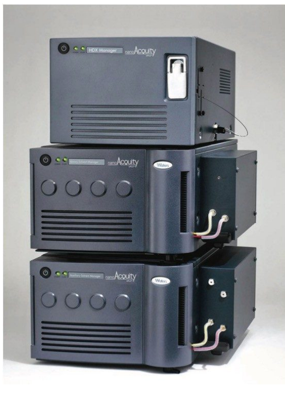
Figure 1. nanoACQUITY UPLC System with HDX Technology. HDX Manager, Binary Solvent Manager (BSM), and Auxiliary Solvent Manager (ASM) are shown from top to bottom, respectively. The HDX Manager is a key component, which can perform the online pepsin digestion and maintain the low temperature at 0 °C required for HDX MS.
