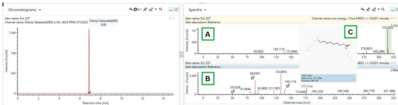
Figure 3. An example of MS^E data for dibutyl sebacate. [A] Low energy spectra with the precursor ion ( C_{18}H_{34}O_4 , exact mass 315.2535, mass accuracy: -1.0 ppm). [B] High energy spectra with the fragment ions. [C] The symbols in the high energy spectra indicate there is an assignment for the fragment ions and the mass accuracy associated with it. The charge retaining fragment is highlighted.
